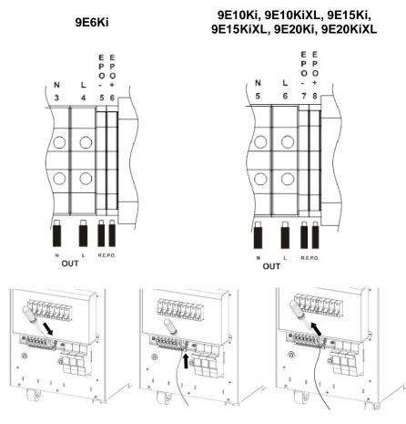
Fig.3-7 EPO terminal connection
