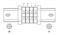
Fig.3-8 EBM terminal view (Fuse for 9E6Ki, 9E10Ki, 9E10KiXLwithout Neutral)
