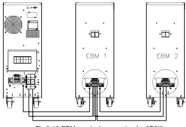
Fig.3-10 EBM terminal connection for 9E6Ki, 9E10Ki, 9E10KiXL With Mutliple EBM
