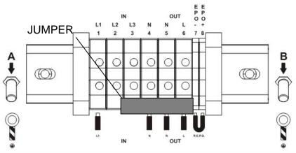
Fig.3-5 10~20K single phase input terminal view
