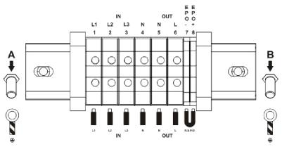
Fig.3-6 10~20K three phase input terminal view
