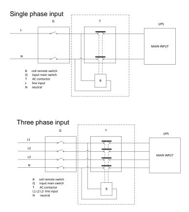
Fig.3-2 Typical external isolating device installation
