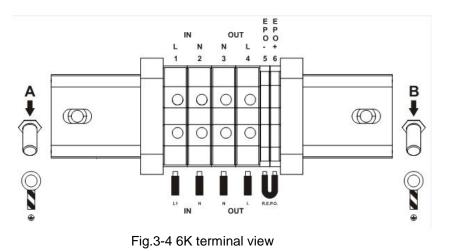
6. Tighten the terminals well, close the backpanel cover and secure it with the screws taken out earlier.
